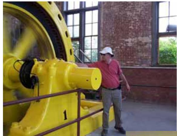
*James Besha demonstrates the stability and lack of vibration of the generator by balancing a nickel on the shaft support.*
